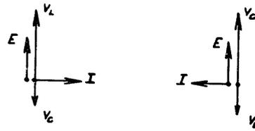
Figure 2 Vector diagram of LC circuit
