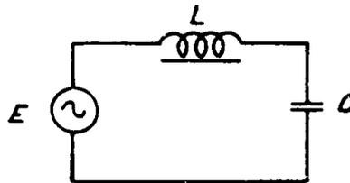
Figure 1 – Typical Ferroresonant Circuit
