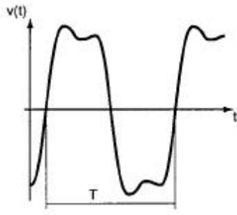
**Figure 5 Fundamental mode of ferroresonance**
