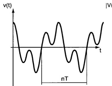
**Figure 6 Subharmonic mode of ferroresonance**
