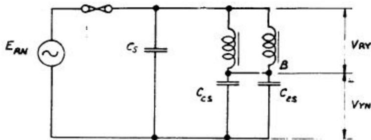
**Figure 10 Single phase equivalent circuit**
