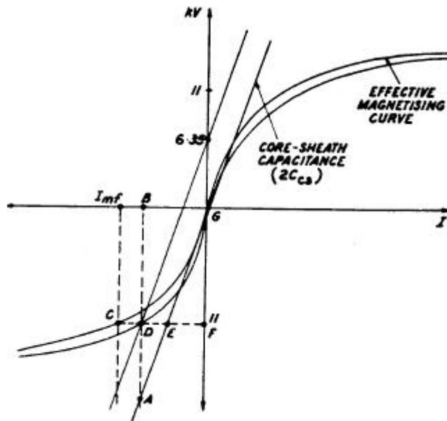
**Figure 20 Critical Cable Length**
