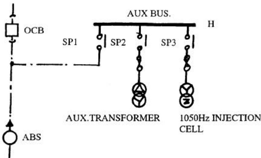
Figure 19 Single phase switching zone sub auxiliary bus with frequency injection cell
