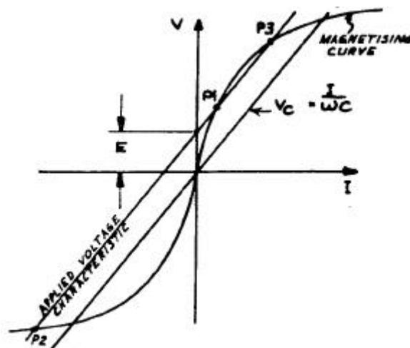
Figure 3 Graphical Construction for Analysis of Circuit
