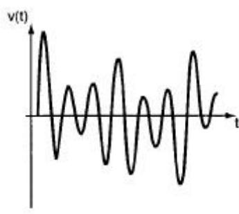
**Figure 7 Quasi-periodic mode of ferroresonance**
