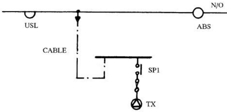
Figure 18 Switch overhead network with tee'd cable to padmount substation
