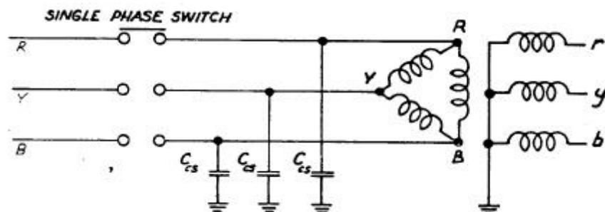
Figure 9 Three-phase equivalent circuit
